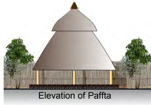
Figure 5.9 Graphical analysis of Paffta vernacular house. Show the Paffta floor plans uses for elders' judge under the shade of Paffta called Weyebeta space and the young unmarried Konso dwellers slipping in the upper floor level called Affda space. There are some explanation for the elevation, section and natural light distribution and pathway in graphical presentation.
