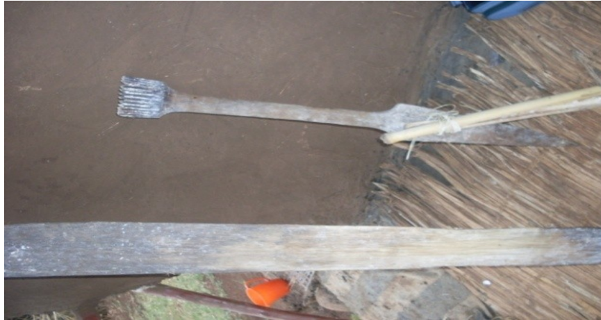
Figure one: - This figure refers to the instruments which enable them to produce ‘qia/q’acha’. watar’ (lit. a flat smooth wood), ‘sisha’ (lit. a thin flat ruler type of stick made of bamboo tree) and ‘zange’ (lit. a tool which is very narrow to the bottom and like fork to the top).
