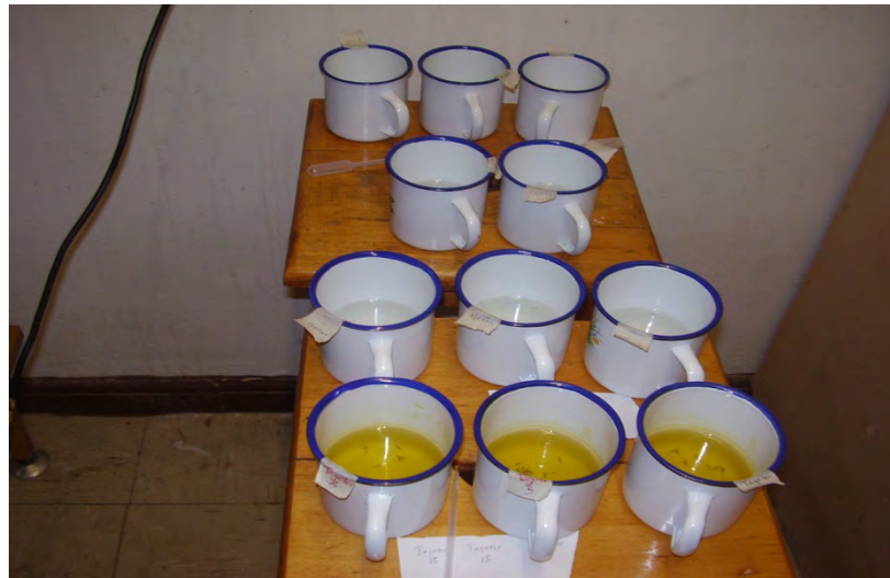
Plate 7. Larvicidal bioassay in the laboratory using white enamel cups
