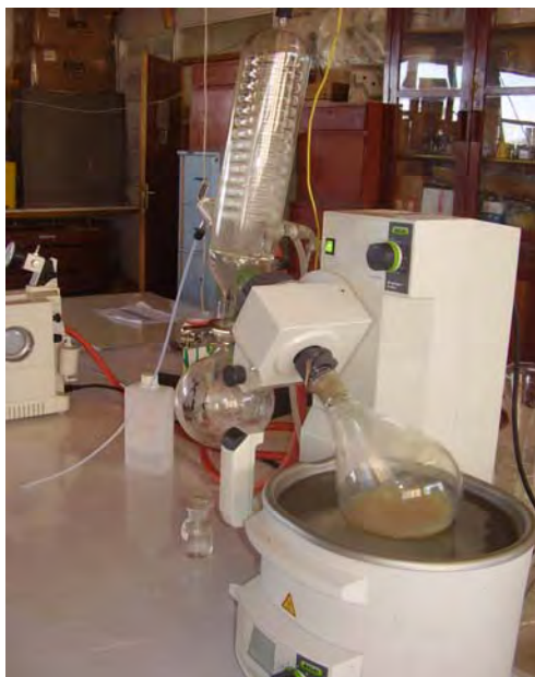
Plate 6. Rotary evaporator apparatus used for solvent extraction
