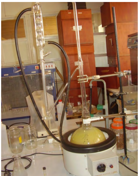
Plate 5. Clevenger type apparatus used for essential oil extraction
