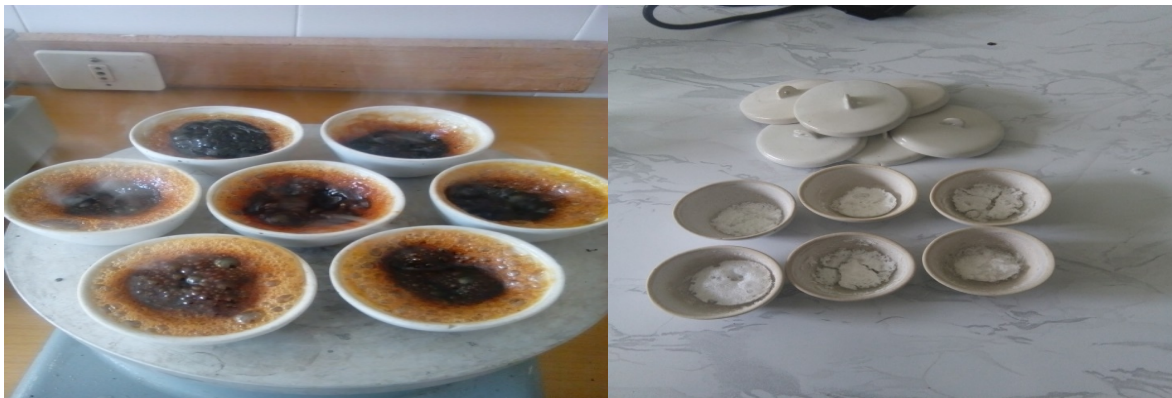
Annex 4: Ash Analysis using muffle furnace ( carbonation of honey samples using hot plate)
