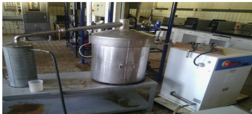
Figure 3.2 Steam distillation of Chemical and Bio engineering of AAiT
