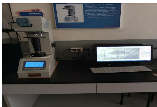
Figure 3.20 Micro hardness test setup
