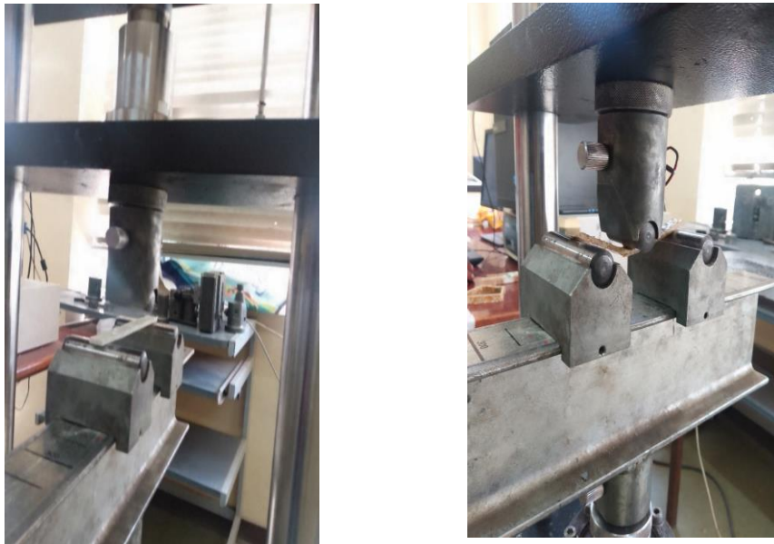
Figure 3.18 Flexural test setup and specimen under bending stress
