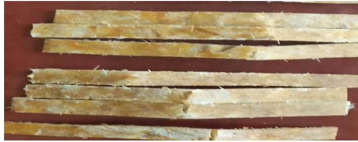
Figure 4.11 Specimens after bending test
