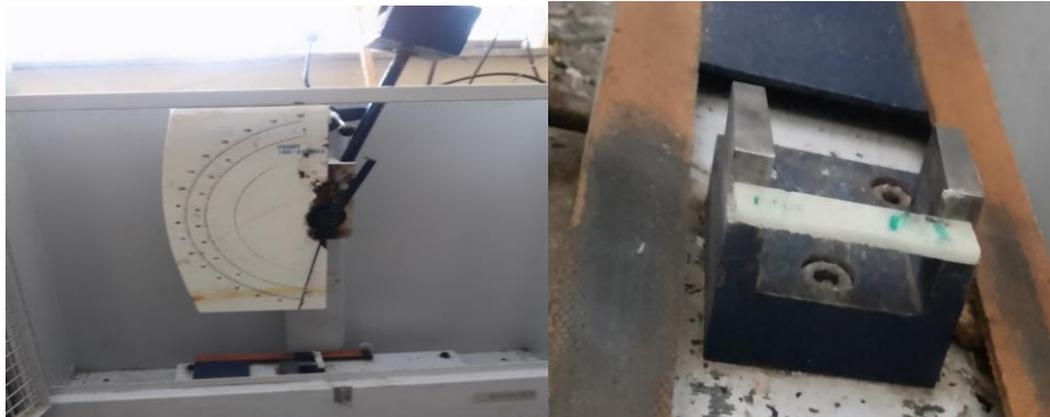
Figure 3.19 Charpy impact test setup and specimen under impact load
