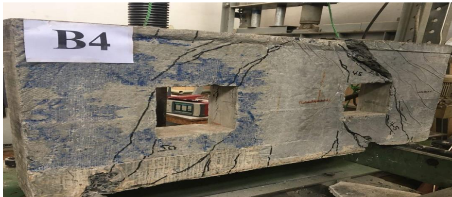
Figure 4-12 Shear failure at the ultimate load
