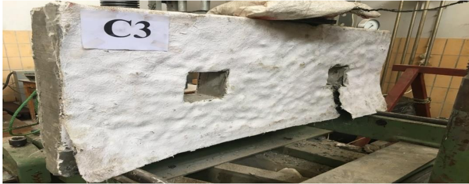
Figure 4-16 De-bonding and rupture of GFRP sheet
