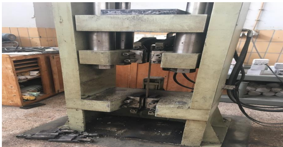
Figure 4-3 Testing for steel bars for tensile strength
