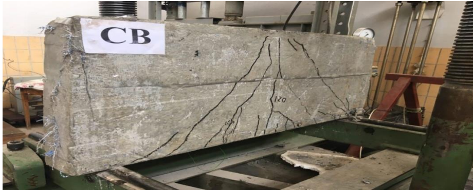
Figure 4-8 Control beam specimen after testing
