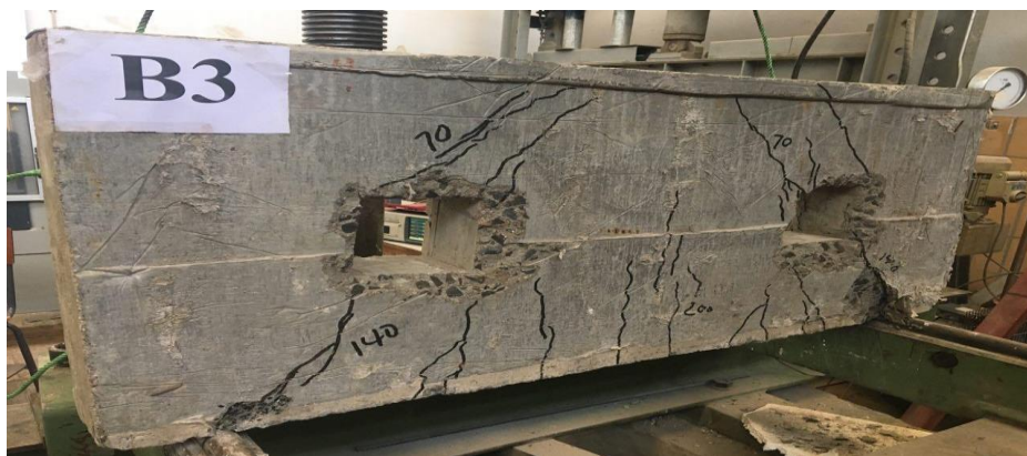
Figure 4-11 Shear and flexural cracks
