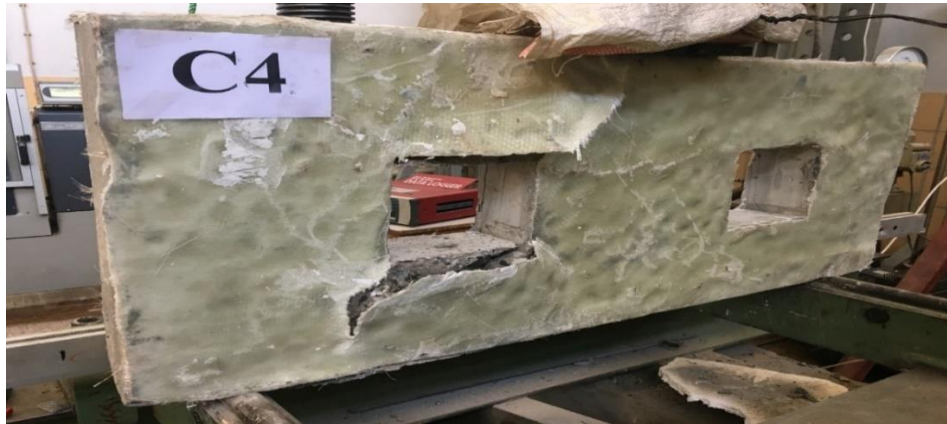
Figure 4-18 De-bonding and rupture of GFRP
