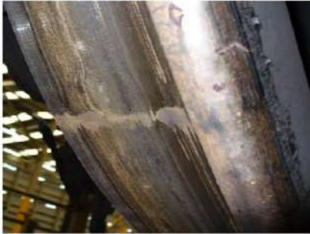
Figure 11: Incorrect mill feed as a result of bad turning [43]
