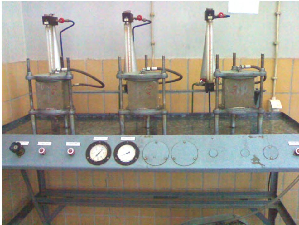
Figure 6.1. Permeability apparatus with samples assembled onto it
