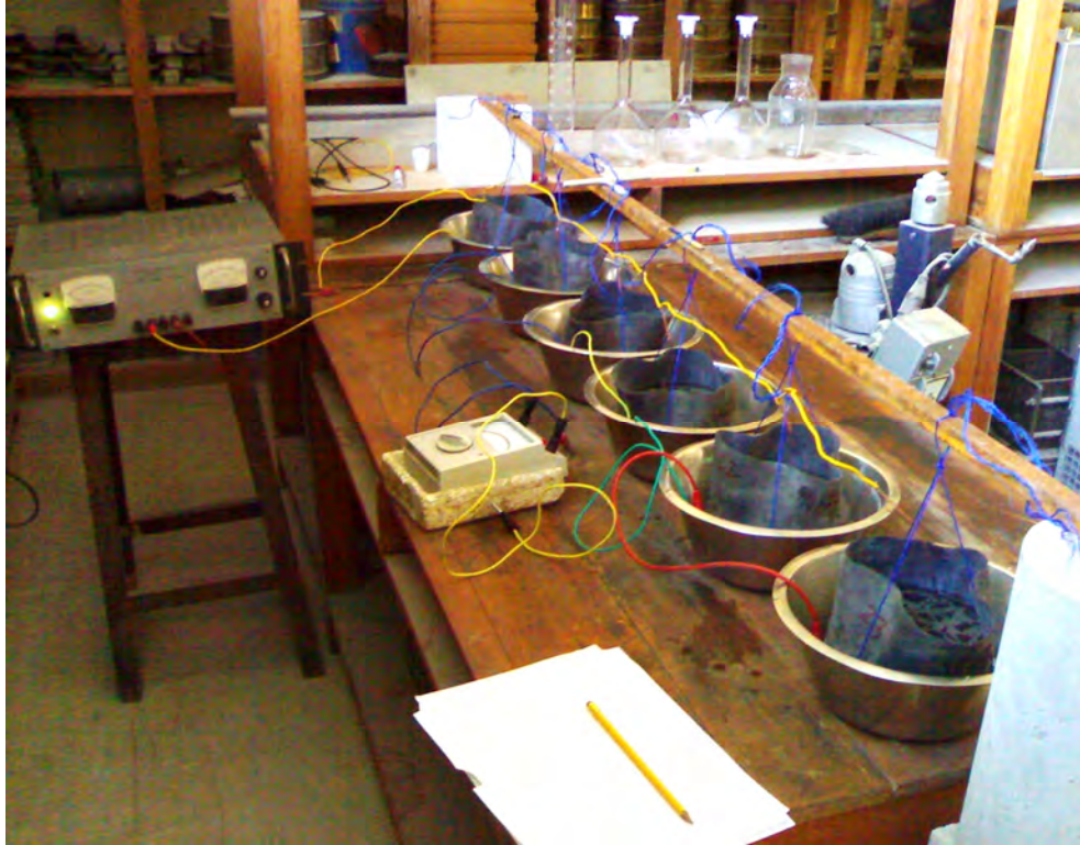
Figure 6.4. Experimental setup used for conducting chloride migration test
