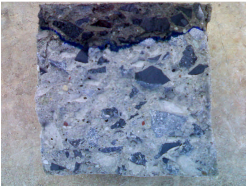
Figure 6.2. Typical concrete sample just after splitting at the end of the water penetration test
