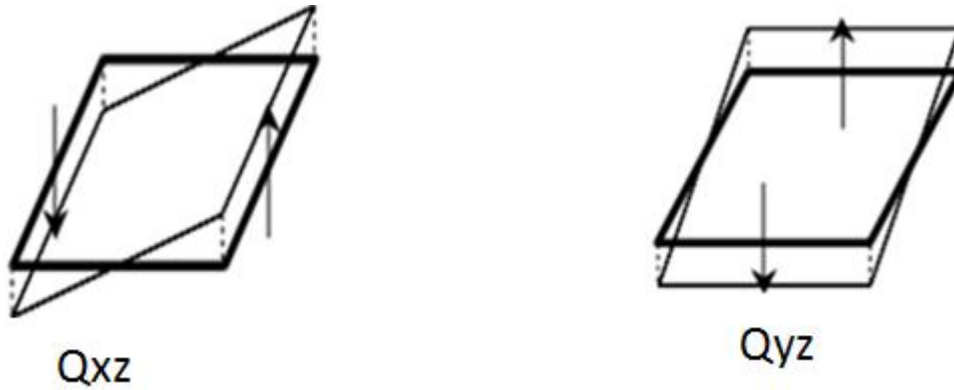
Figure 4. 8: Definitions of positive shear forces per the local axes given in Figure 4.7.
