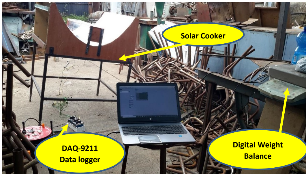
Figure 5.12: Testing arrangement of the tube type direct solar oven
