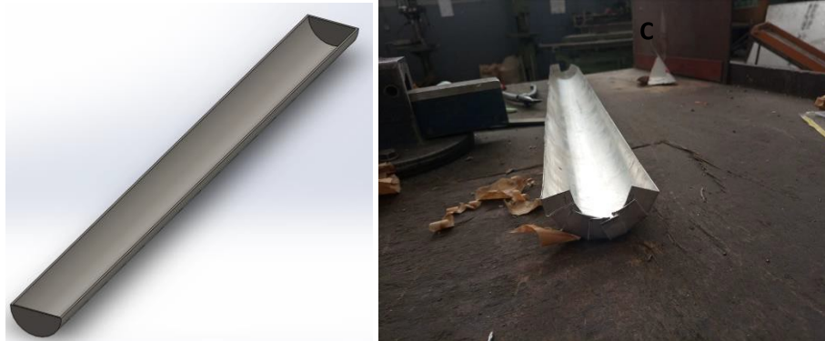
Figure 5.8: Sliding tray SOLIDWORKS and manufactured prototype
