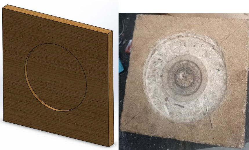
Figure 5.3: End seal drawing and manufactured part
