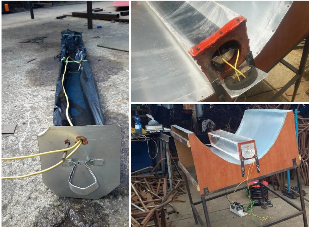
Figure 5.11: Thermocouples passed through oven door and placed inside oven
