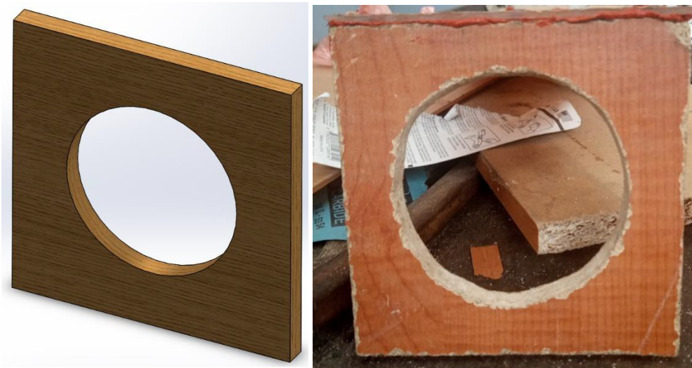
Figure 5.2: Front seal drawing and manufactured part
