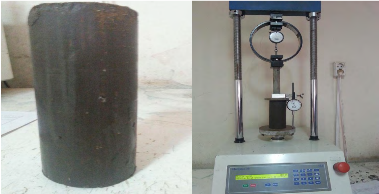
Figure 22: UCS tests in the Laboratory
