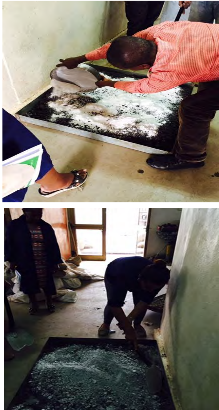
Figure 20: Mixing of Soil and Stabilizer in the Laboratory
