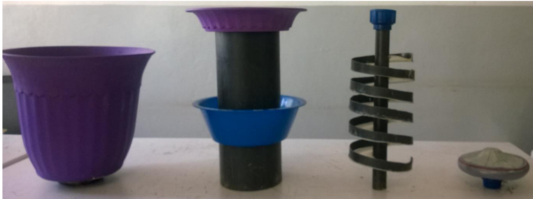
(a) Exterior part or System holder (b) The inner part or Filtration media (c) Filtration channel (d) Deflector
