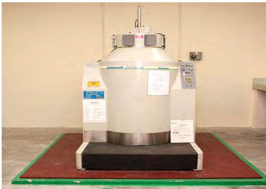
Fig.1. Diagram of ^{60}\text{Co} Gamma Cell- 220 Excel Nordion MDS India (Naboletal 1998).
