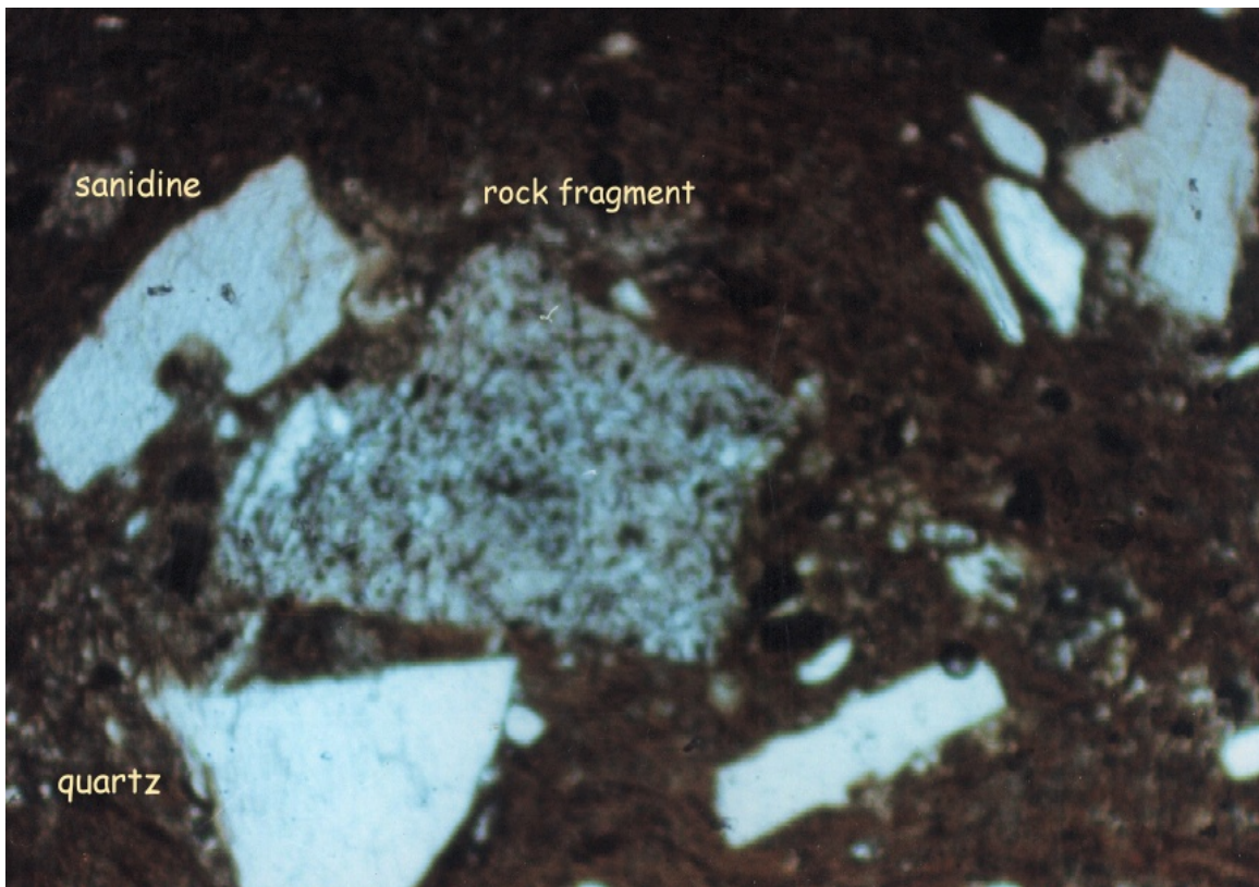
Figure 4.10 Crystals (sanidine and quartz), and rock fragment at, 5X magnification and PPL in GUN-22
