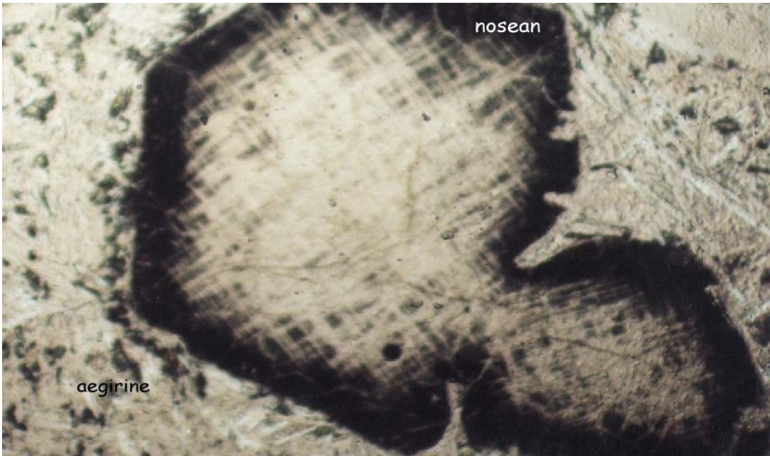
Figure 4.15: Phenocryst of nosean at, 5X magnification and PPL in GUN-36
