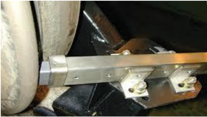
Figure 3.11 Old or existing AALRT train lubrication system
