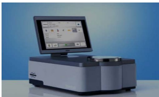
Figure 7: FT-Near Infrared Spectrometer (Tango, Bruker Optics GmbH, Germany).
