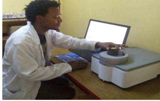
Figure 12: Scanning samples for spectral Data Using Tango FT-NIR Spectrometer
