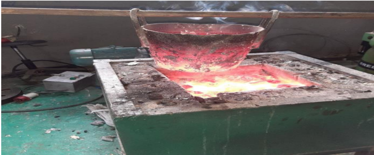
Figure 3. 13 Taking the molten material for pouring As shown in figure 3.13 the molten hybrid material ready to pouring in to the prepared mold
