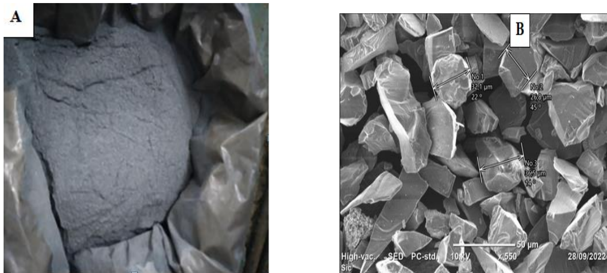
Figure 3. 1 Silicon carbide (A) powder (50µm), (B) morphology of SiC(conducted at ASTU)
