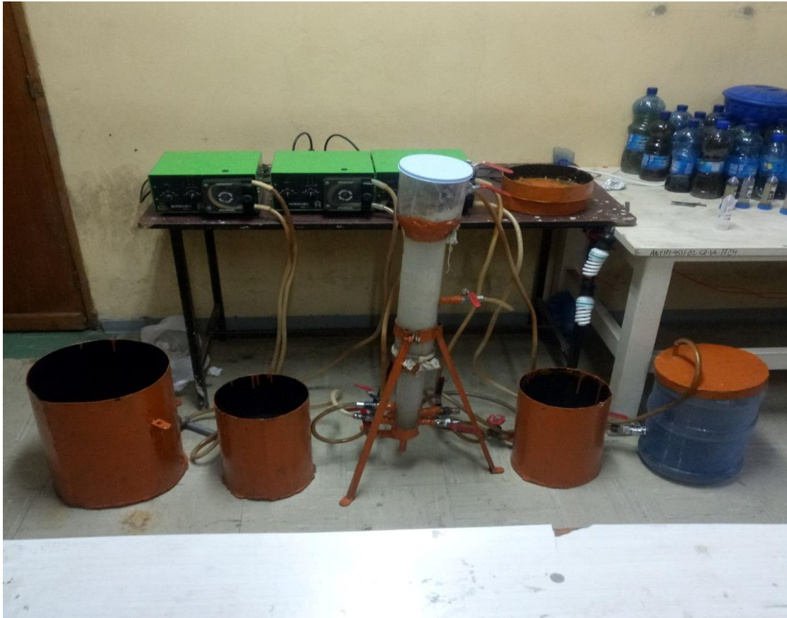
Figure 1 Fluidized bed reactor with cone and whole FBR systems
