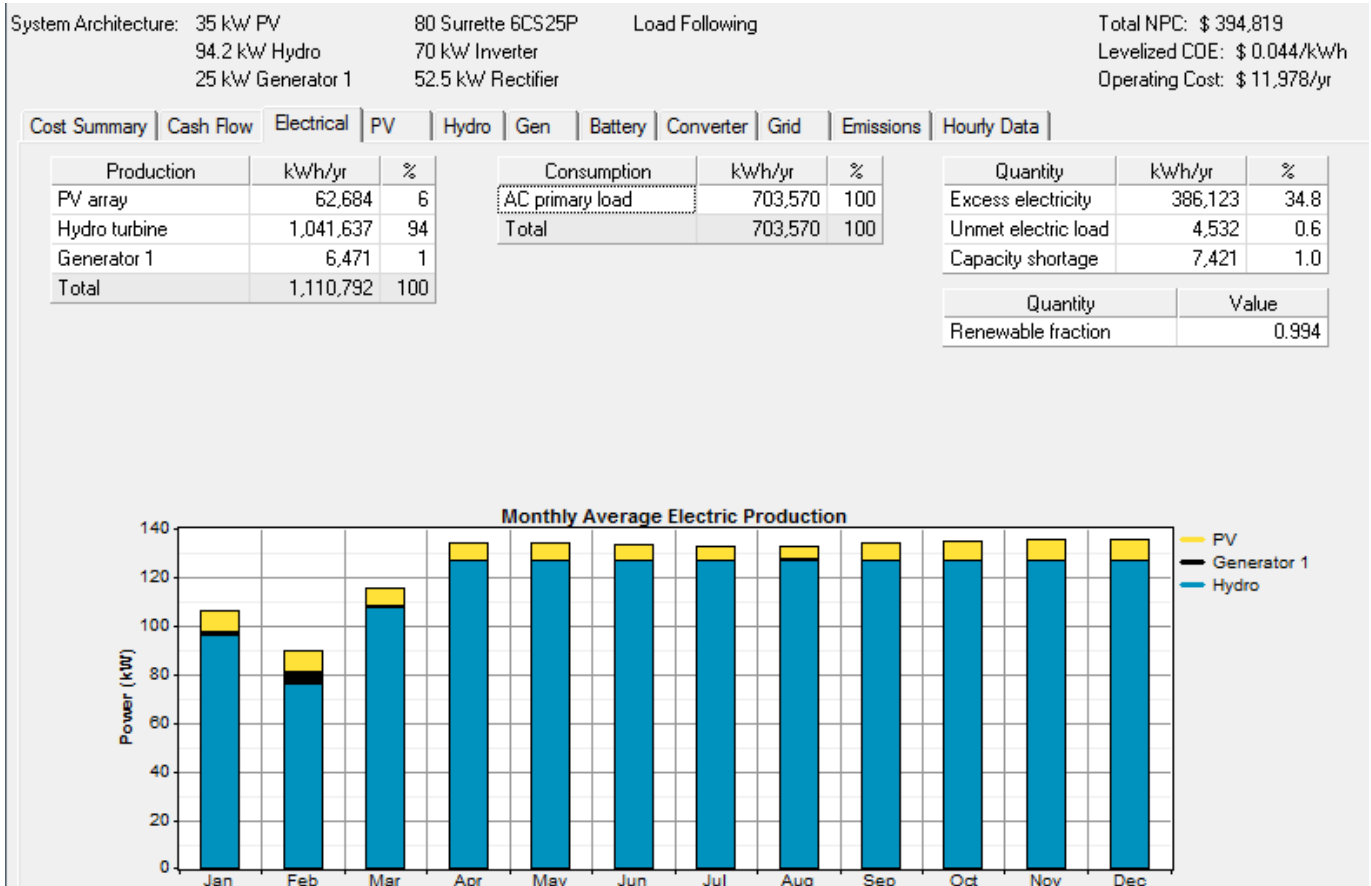
Figure 7.6: System architecture and monthly average electric production
