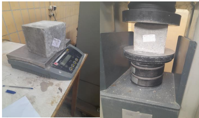
Fig. 3-1 Compressive strength test of concrete
