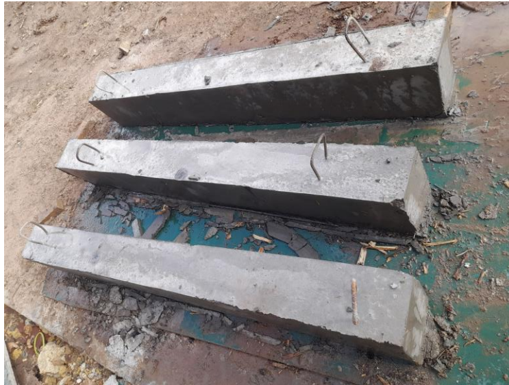
Fig. 3-12 Beam specimens after dismantling formwork
