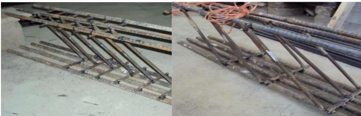
Fig. 2-2 Single and legged swimmer bar respectively [11].
