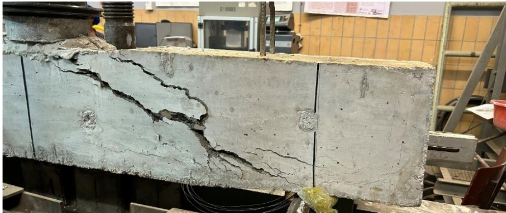
Fig. 5-9 Right Front side of TBNS specimens After failure
