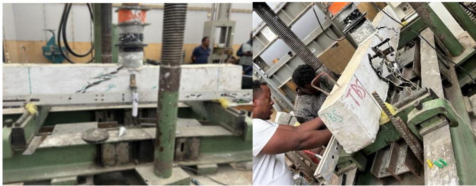
Fig. 5-12 Back and Front side of TBS specimens After failure Respectively
