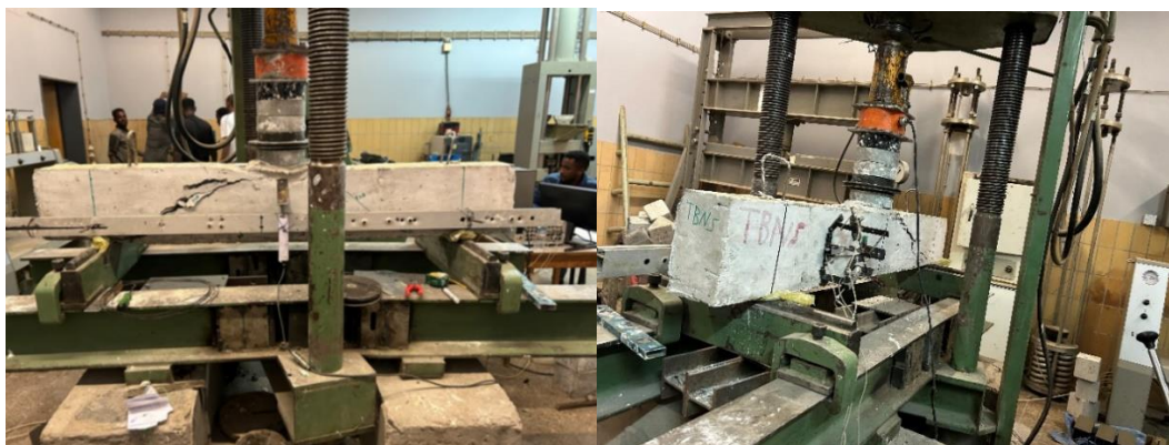
Fig. 5-7 Back and Front side of TBNS specimens After failure Respectively
