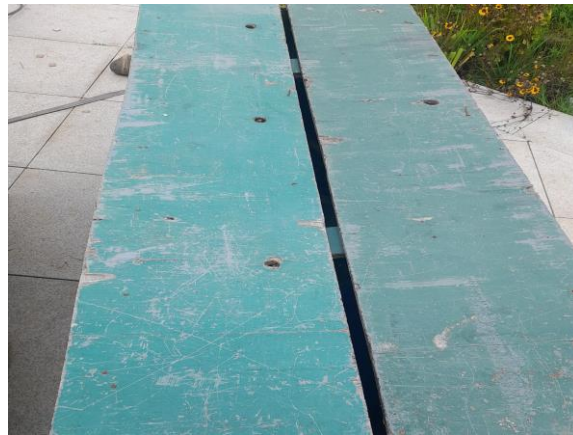
Fig. 3-3 Wood-plastic composite formwork
