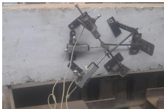
Fig. 3-15 Transducers attached on beam surface
