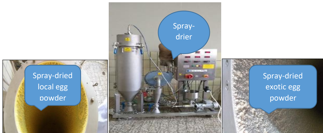
Figure 4: Spray dryer used to make whole egg powder
