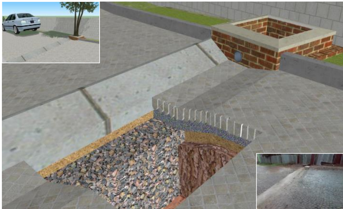
Figure 6: 3D-Illustration of the proposed design for on-site management of stormwater runoff from cobblestone streets, referred to as ‘Infiltration Bumper with Tree Planter’
