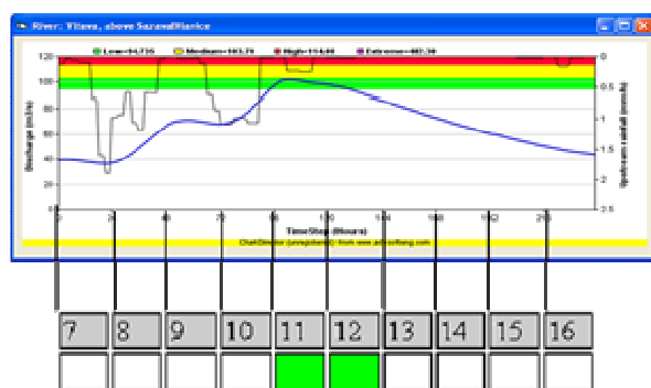
Figure 2.6 Single deterministic forecast result (Source: EFAS training material)
