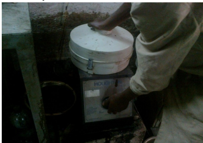
Figure 3-7 Laboratory extraction of asphalt and aggregates
