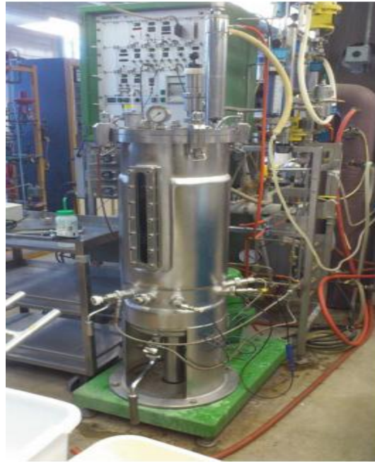
Fig. 2.3 Cultivation of bacteria for biocement production in 50 L fermenter (photo taken at the Fermentation Facility, Iowa State University, USA)
