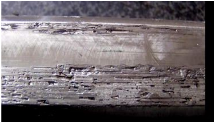
Fig. 2. 2. Scratches causing rail wear [33]
