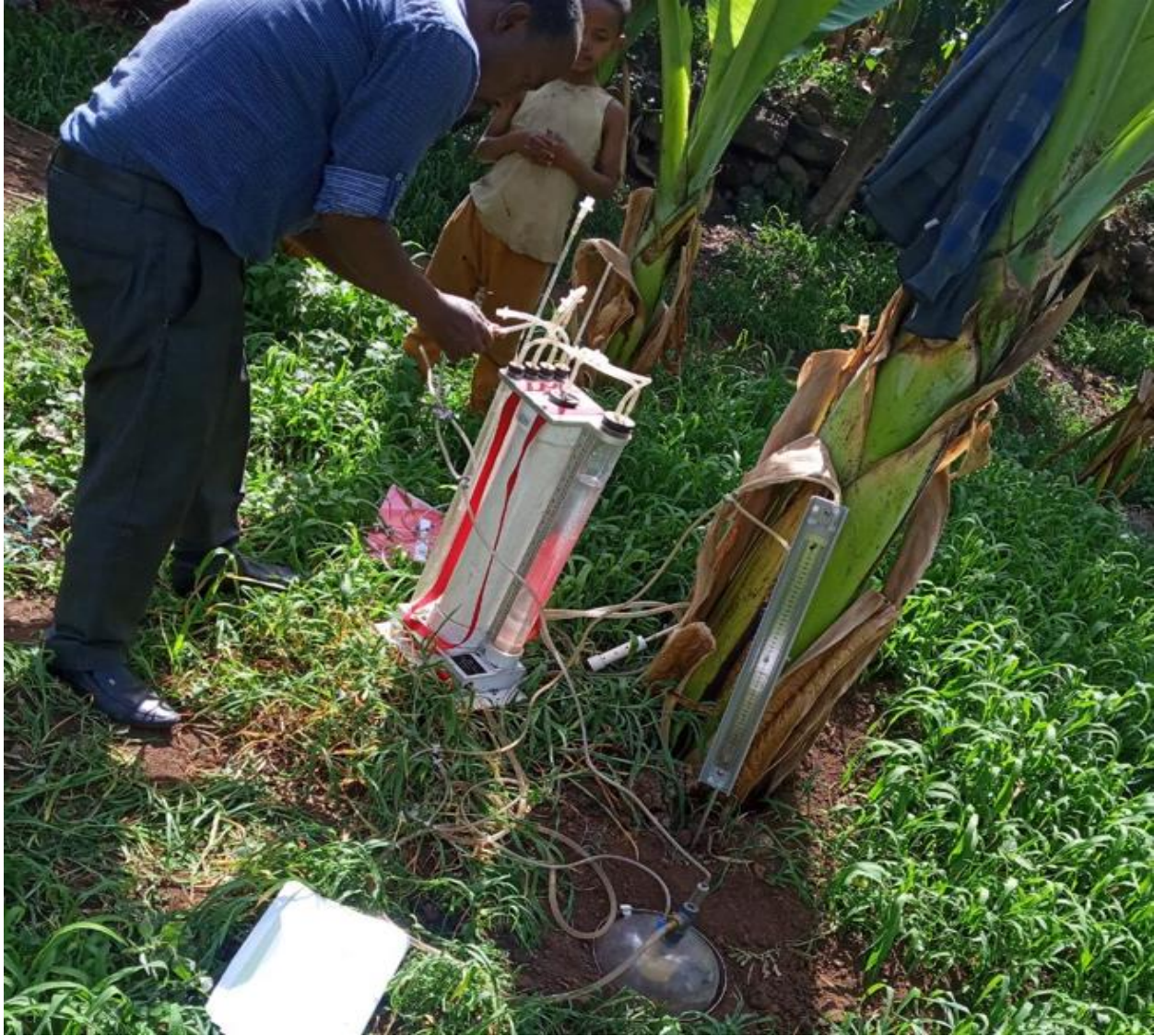
Figure 3-22: Amozimeter (Hood infiltrometer) infiltration rate measurement of EBLUS
