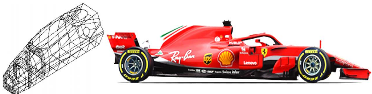
Figure 1.6 Monocoque structure [3] and Formula 1 racing car
