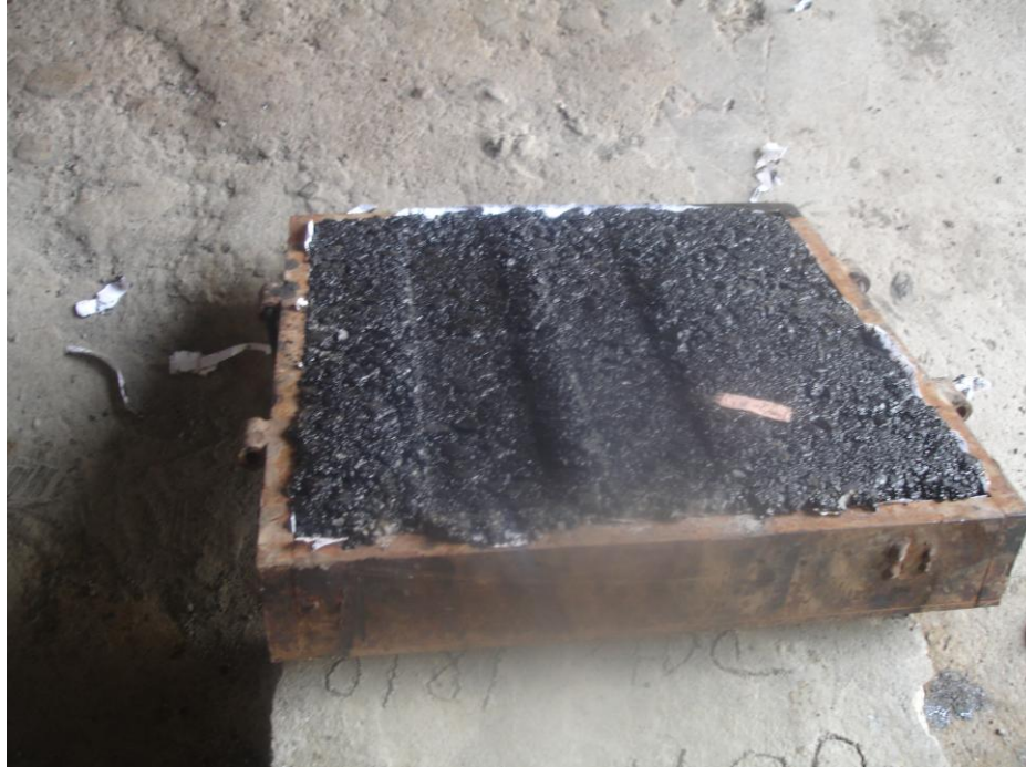
Figure 4.4 Sample After QZDCZSY Testing, 60/70 Binder Grade
