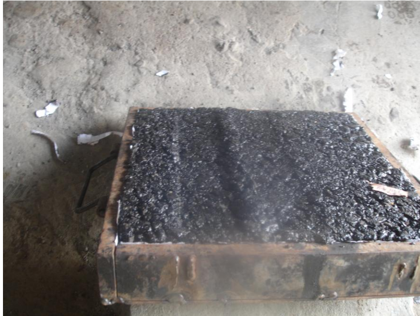
Figure D.2 Specimen with 60/70 Binder Grade and Modifier
