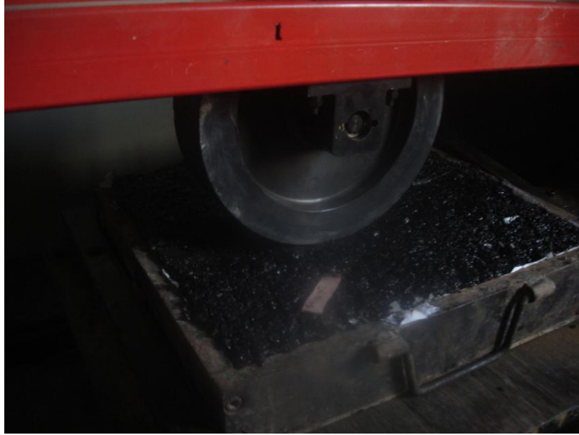
Figure D.2 Specimen with 60/70 Binder Grade and Modifier
