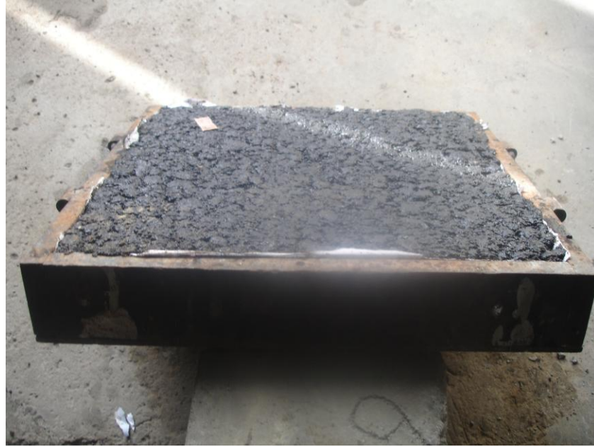
Figure D.4 Specimen with 40/50 Binder Grade and Modifier
