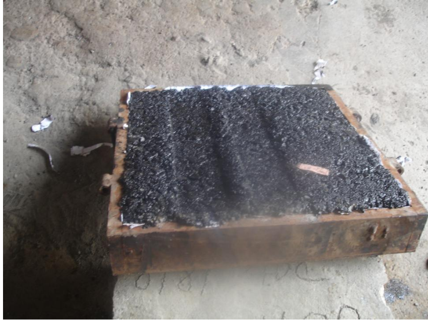
Figure D.1 Specimen with 60/70 Binder Grade
