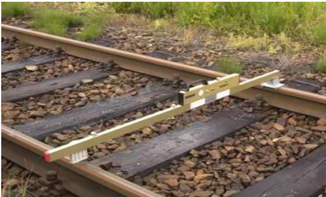
Figure 3.3: Gauge ruler for measurement of track geometry(Francis, 2018)
