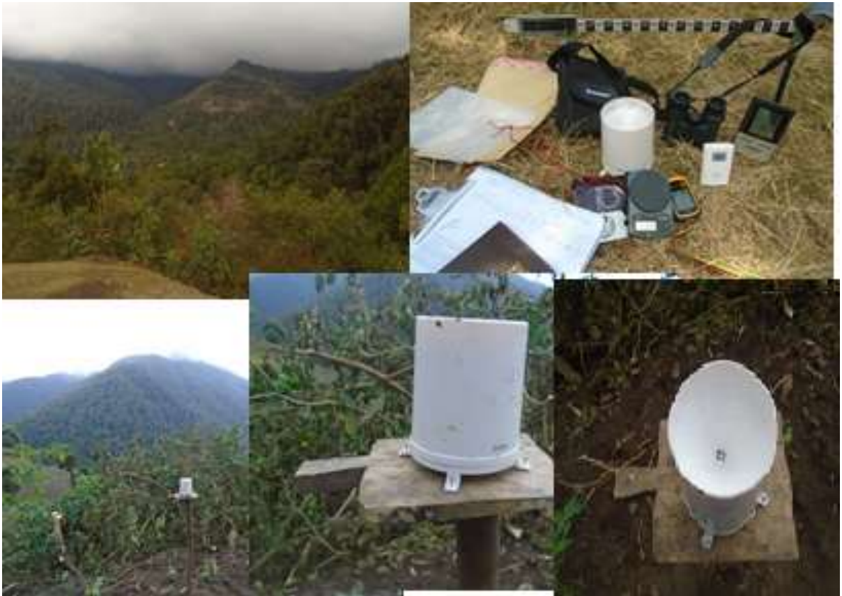
Plate 2. Photos of field equipment and installation of Oregon wireless rain gauge and Taylor digital water proof maximum/minimum thermometer (Source: Dereje Yazezew, 2015).
