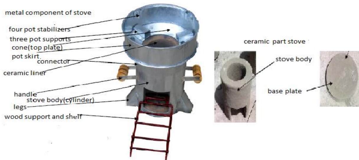
Figure 3.1 Component of tikikil stove
