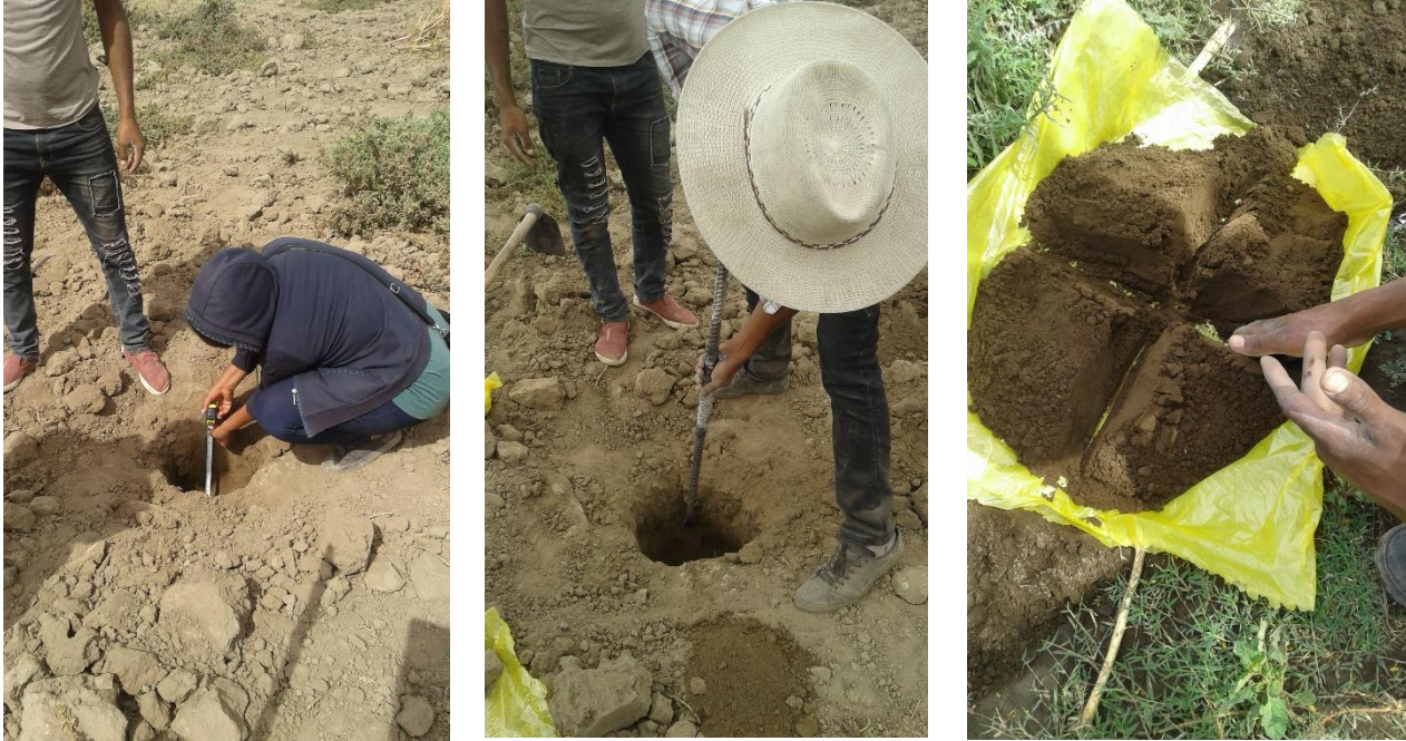
Figure 3.2: Soil sampling techniques at different depth
