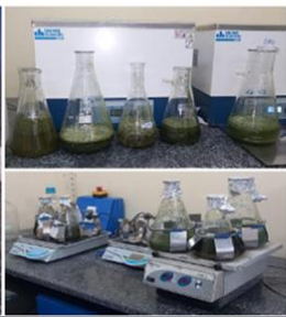
Shaking the crude extracts using Orbi Shaker at 158 rpm
