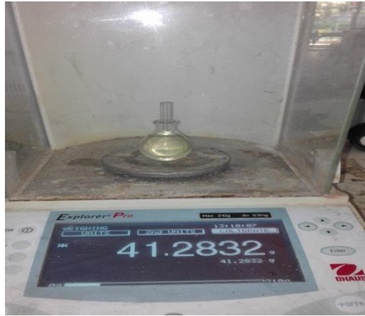
Figure 3.4. Density measuring using pycnometer
