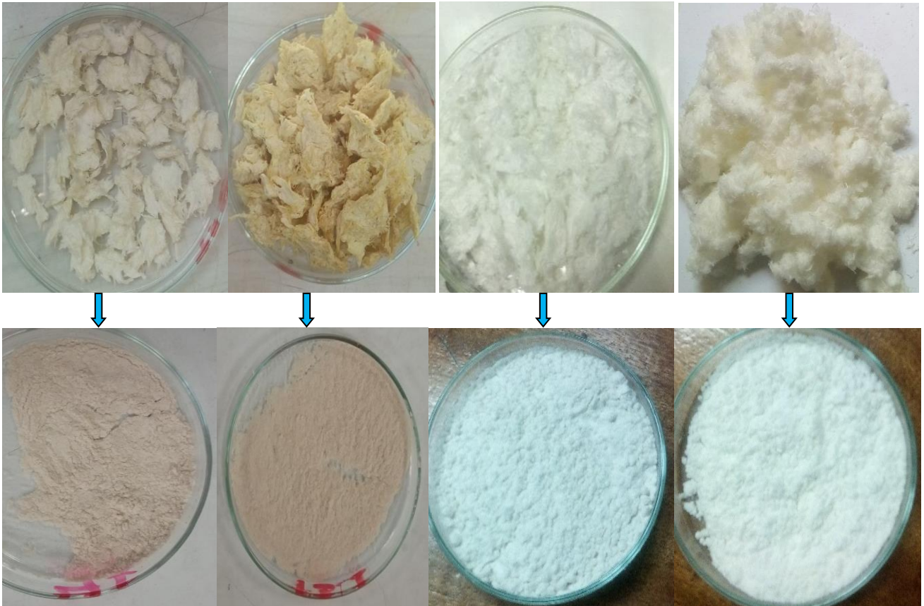
Figure 3: Cellulose (top) and MCC (bottom) isolated from Teff straw following alkali & steam, hot water, formic acid, and formic/acetic acid (left to right) treatment.
