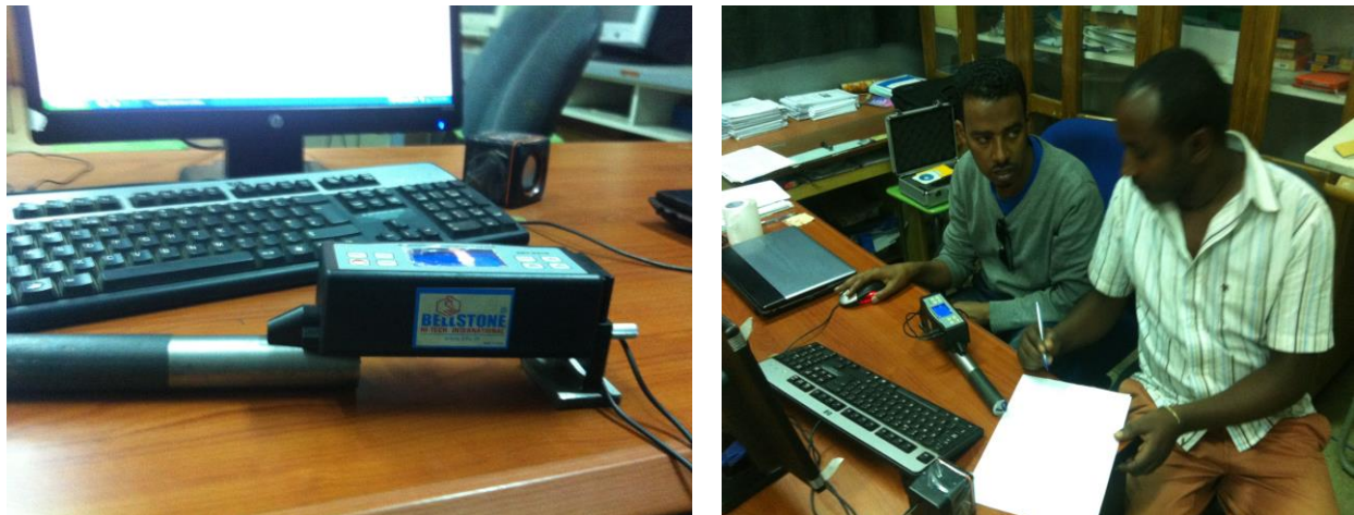
Fig 3.4: Photographic view Bell Stone during surface roughness measurement
