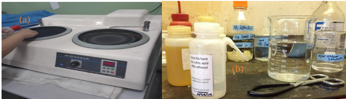
Figure 3-15: (a): polish machine (b): echant
