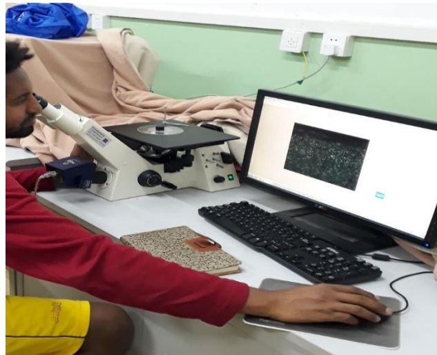
Figure 3-16: Optical Microscope (OM) on microstructure analysis
