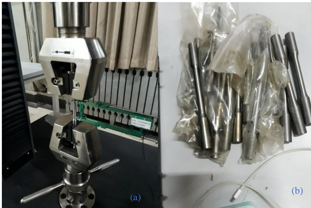
Figure 3-8: (a): universal tensile test machine (b): prepared specimens of the tensile test
