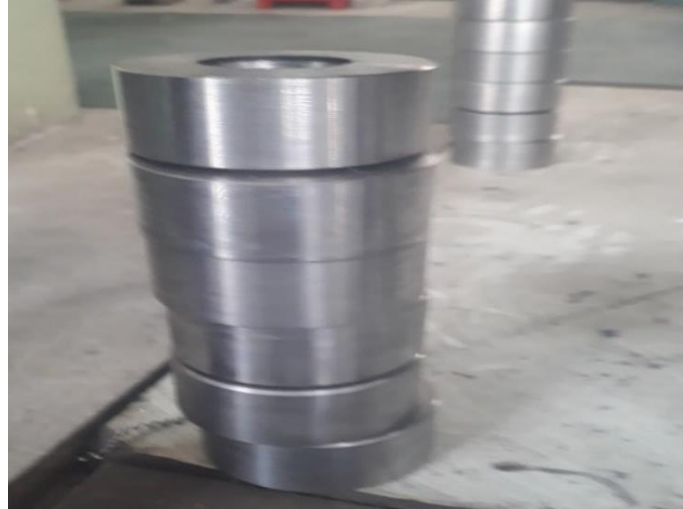
Figure 3-19: EDM finished specimens
