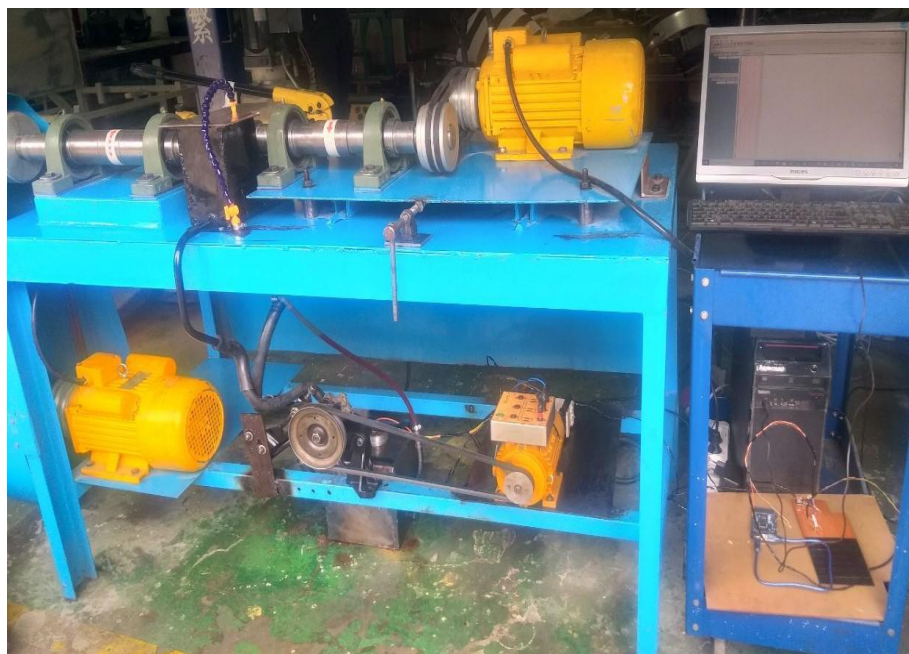
Figure D-10: Final assembled of twin disc RCF test rig
