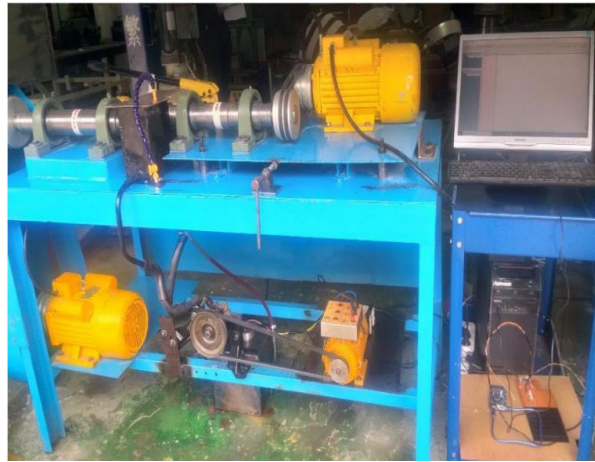
Figure D-9: Assembled load application mechanism
