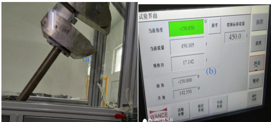
Figure 3-11: (a): Charpy impact tester machine (b): machine specification
