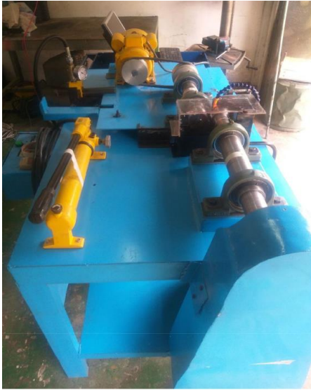
Figure D-9: Assembled load application mechanism
