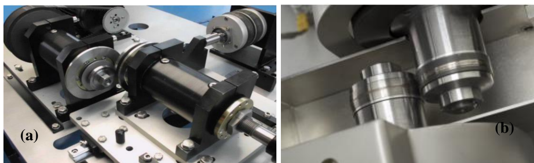
Figure 2-19: (a) TE-72 two- roller test rig: (b) Optimal Instruments test rig [163]
