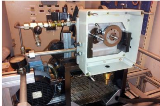
Figure 2-20: Swerea KIMABs twin-disc test rig [163]
