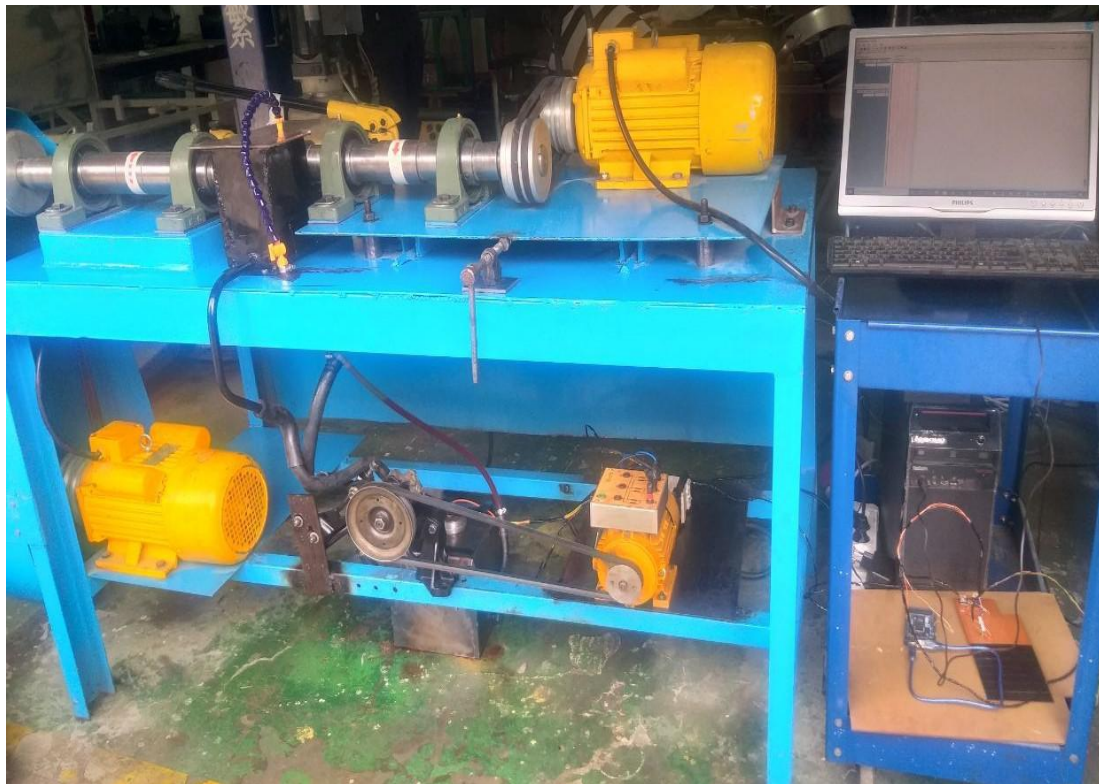
Figure 3-20: Adapted twin-disc test rig
