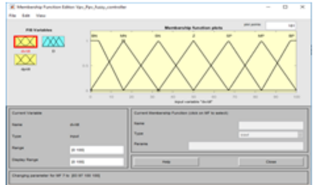
Fig. C.2 Membership function r input variable (dVpv).
