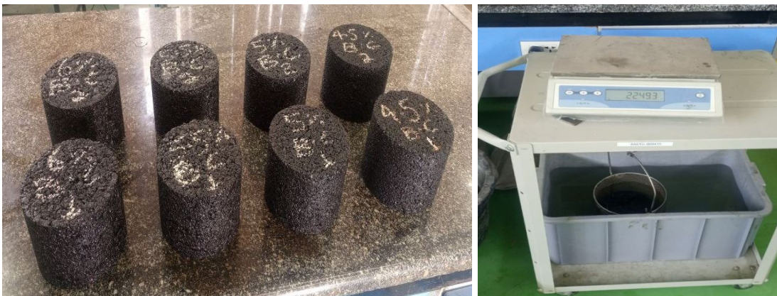
Figure D.15 bulk specific gravity ( G_{mb} ) test for compacted asphalt concrete mixture
