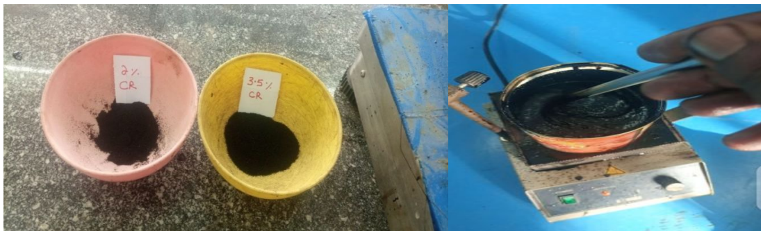
Figure A.2 sample and mix preparation for crumb rubber (CR) modification of binder
