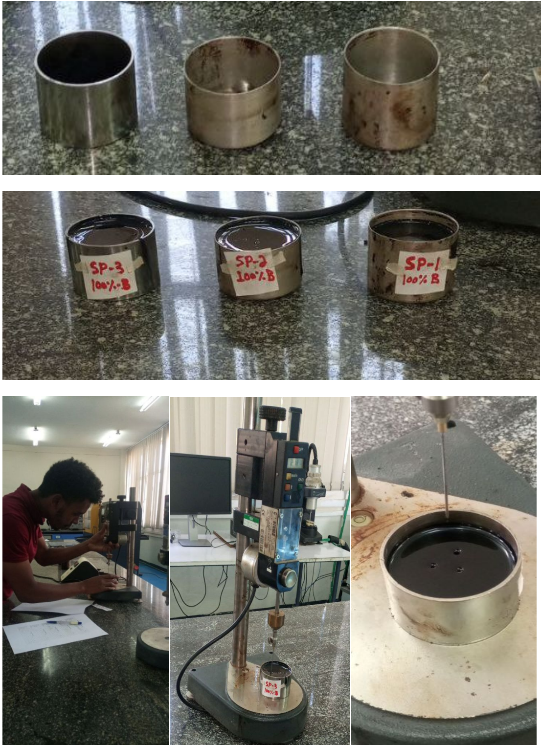
Figure A.3 Penetration testing
