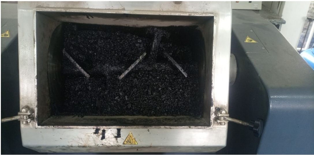
Figure D.9 Aggregate and bitumen mixing
