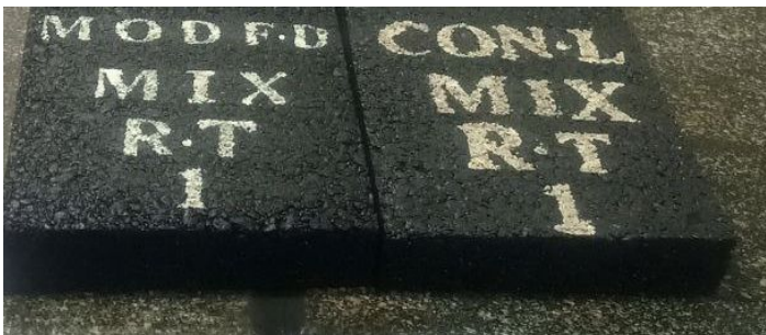
Figure D.17 asphalt concrete slab produced samples for rutting test
