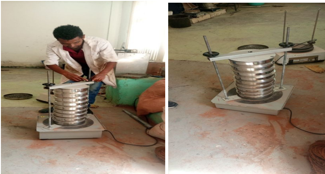
Figure D.6 Aggregate gradation test
