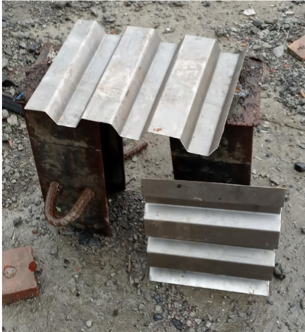
Fig 3.7): EGA 600 cold formed profiled sheet
