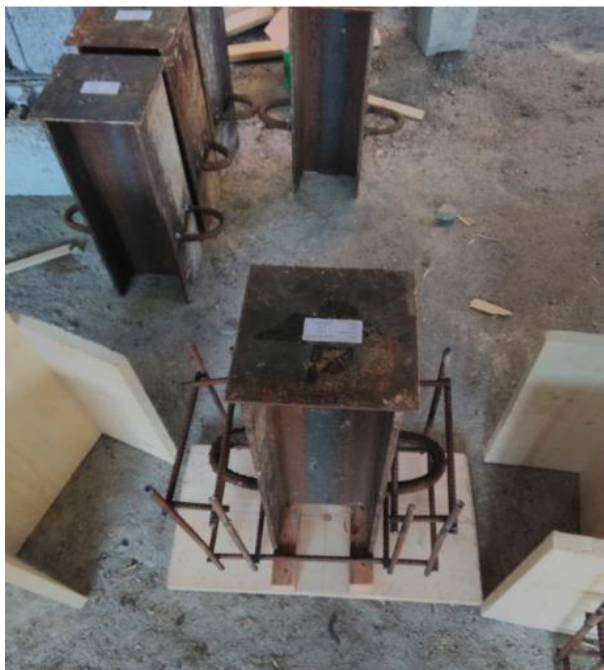
Fig 6.2): 10mm diameter transverse reinforcement welding at intersection
