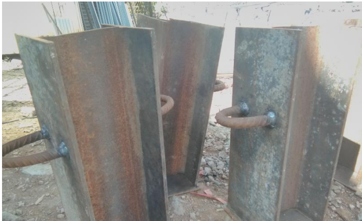
Fig 1.3): reinforcement bar shear connector with hoop shape
