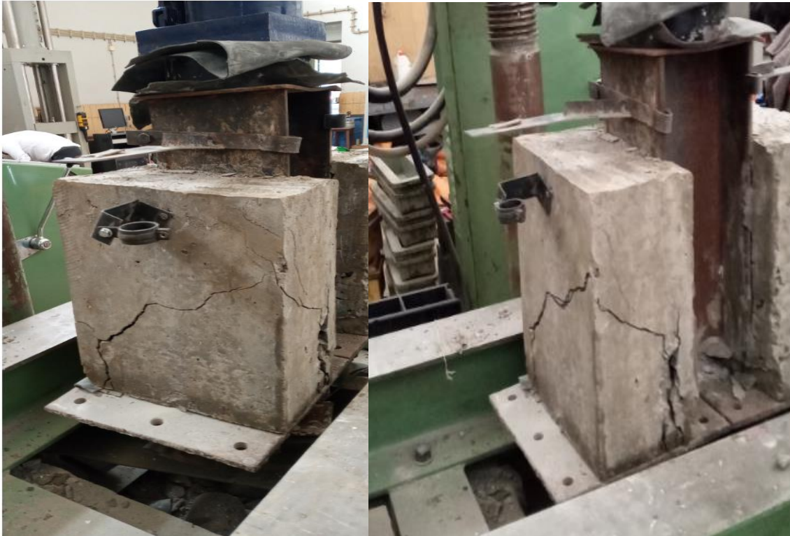
Fig 4.6): failure mode of Specimen S-A-1
