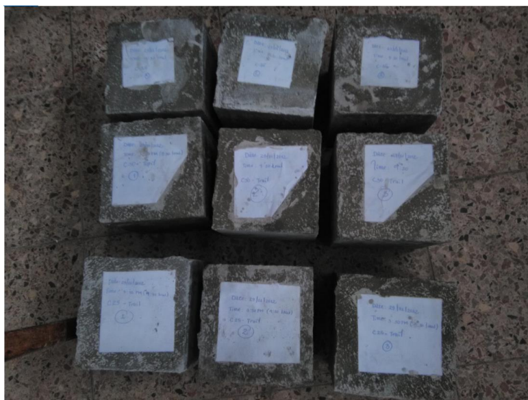
Fig 3.5): Cube test for concrete strength determination
