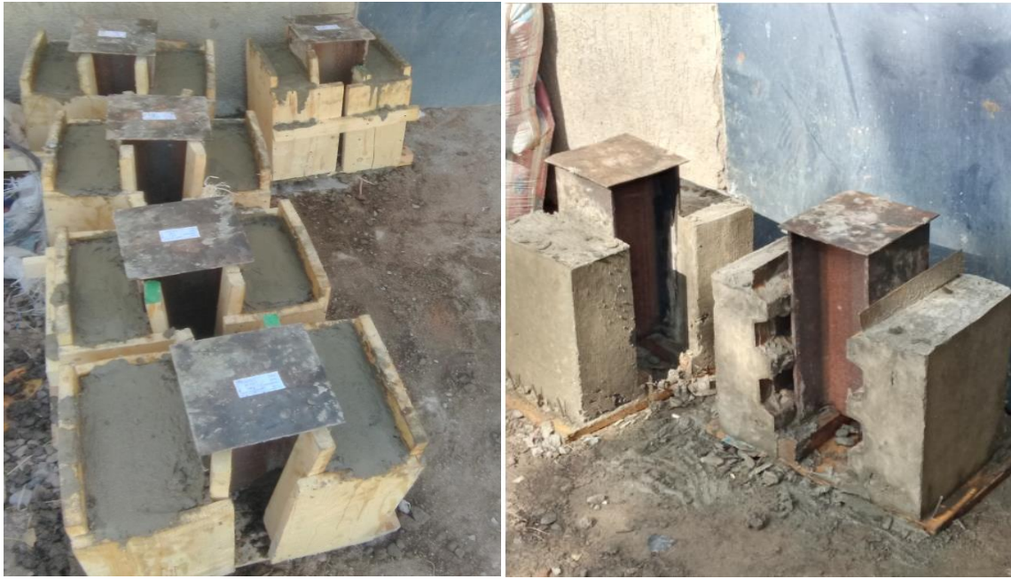
Fig 6.7) specimens after casting of concrete
