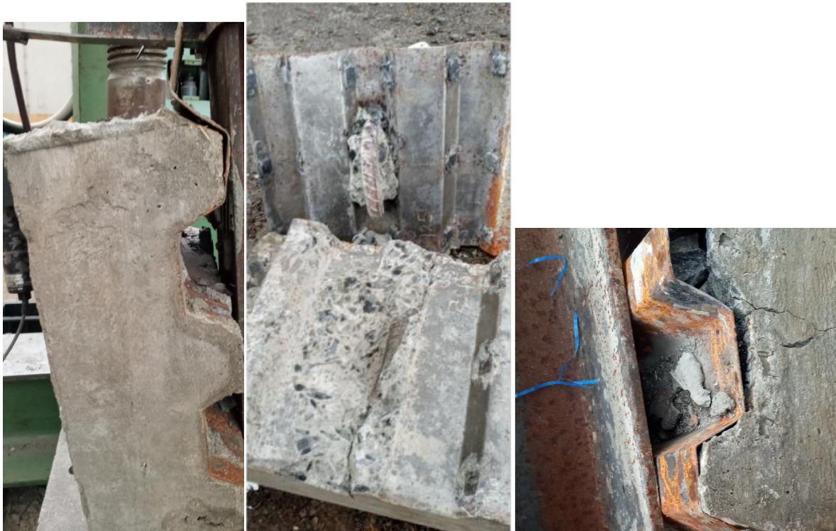
Fig 4.9): failure mode of Specimen S-P-4
