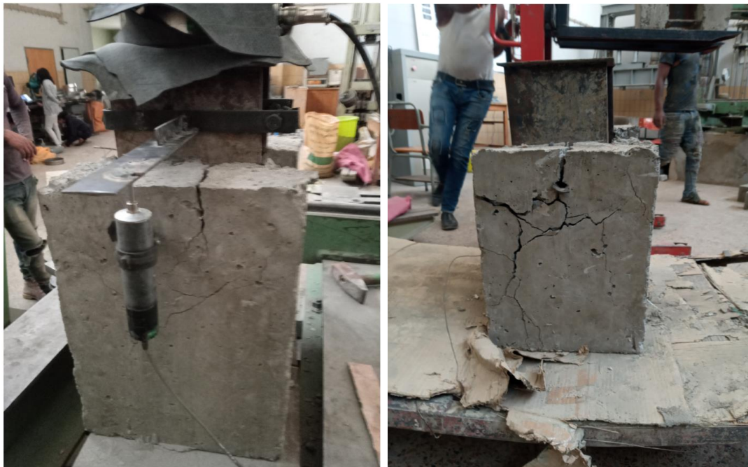
Fig 4.11): failure mode of Specimen S-T-6
