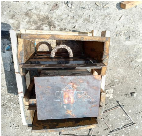
Fig 6.4): formwork preparation for composite concrete slab with single layer of wire mesh
