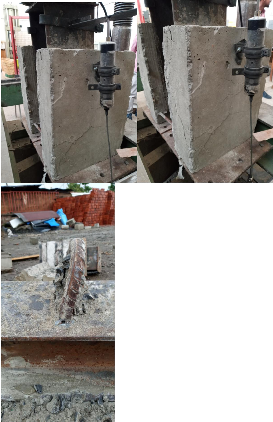
Fig 4.8): failure mode of Specimen S-C-3
