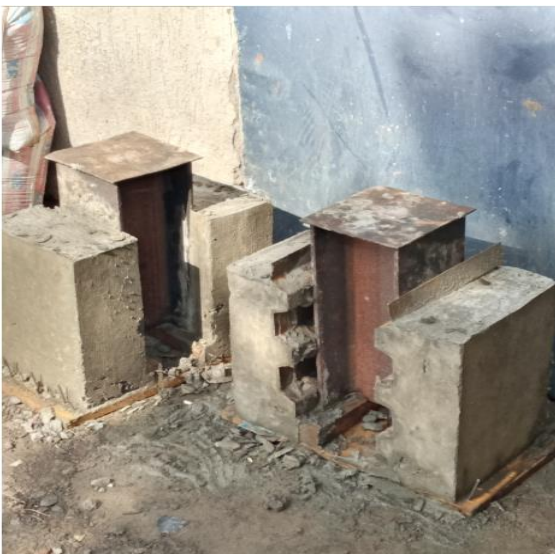
Fig 3.8): formwork preparation for solid concrete
