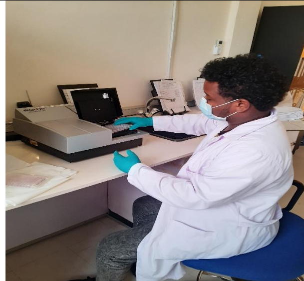
Picture 7: Placing the incubated microplate in microstation reader
