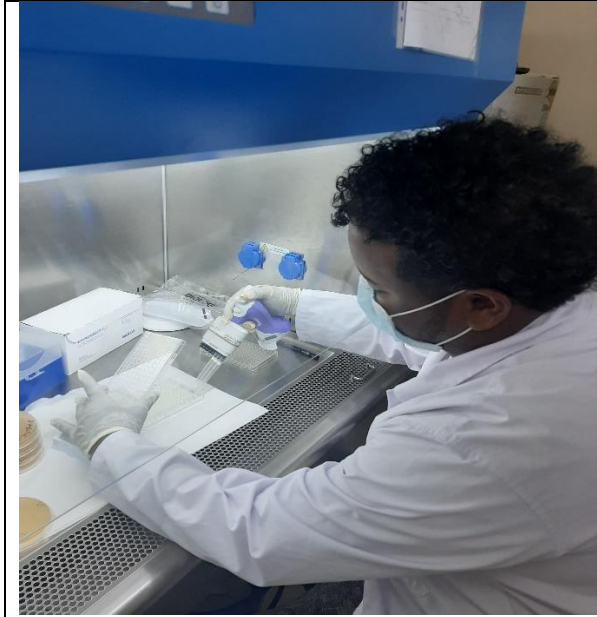
Picture 5: Inoculating the emulsified solution from IFA to the GEN III microplate
