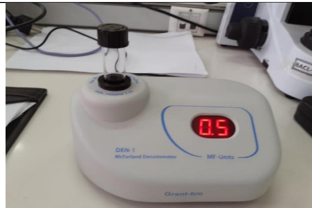
Picture 10: McFarland Densitometer used for checking turbidity during antimicrobial testing
