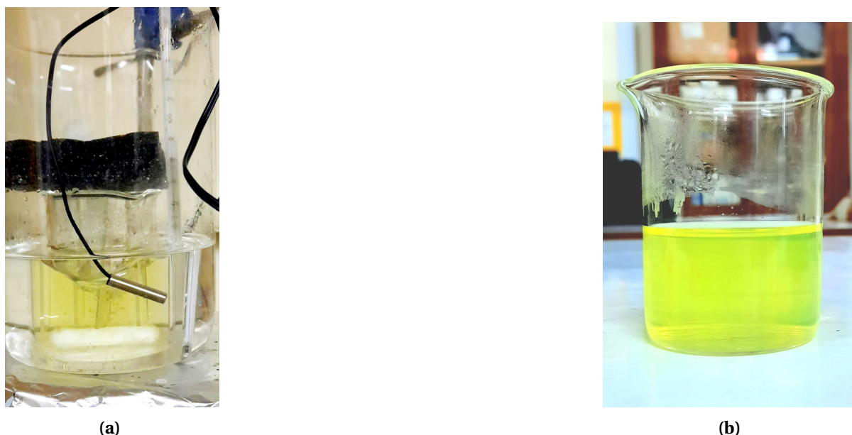
Figure 3.8: (a) CBD process for the synthesis of CdS Colloidal Quantum Dots [The black wire is a thermocouple connected to digital thermometer] (b) As-prepared Pure CdS Colloidal Quantum Dots
