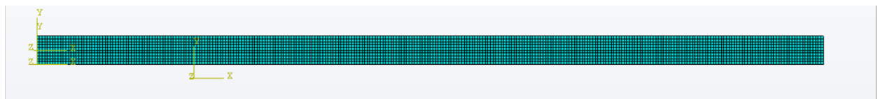
Figure 3.7 Crating mesh with 4-node bilinear plain strain quadrilateral element with approximate meshing size 0.5 mm.
