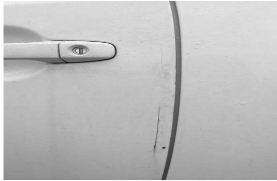
Figure 1.4 A car with a crack on the door of GFRP composite material.[19]
