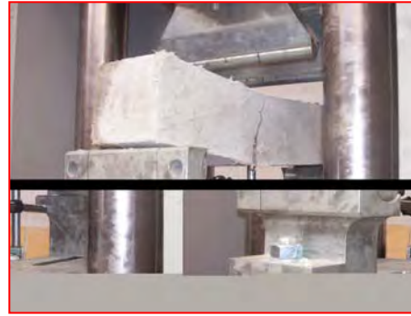
Plate (b) Failure at 1.00% Jute fibre
