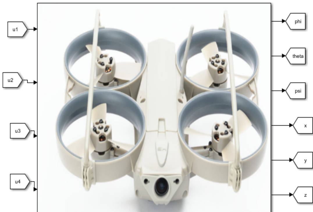
Figure 3.6: Complete Model of Quad-Rotor Dynamics
