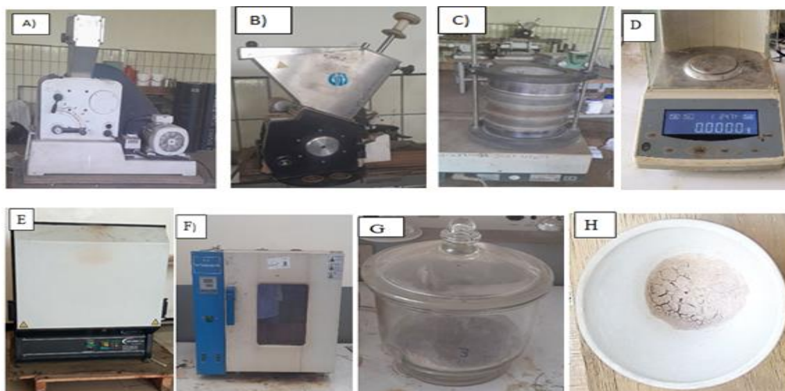
Figure 9: Used laboratory equipment: A) Jaw crusher, B) Hammer mill, C) , Sieve shaker, D) Electronic balance, E) Muffle furnace, F) Universal hot oven, G) Desiccator, H) Silica crucible
