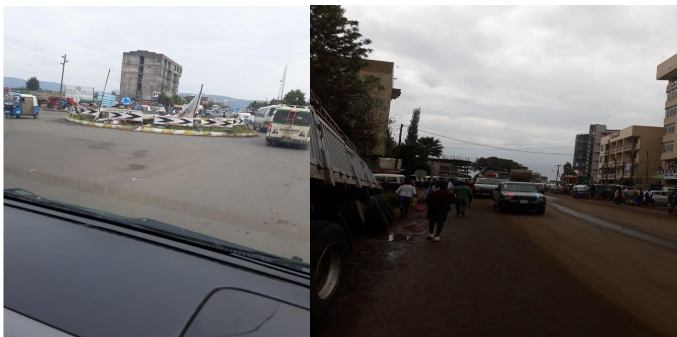
Figure 4.26: Deficient Geometric Design, Lack of Pedestrian Walkway, Lane and Crossing Marking
