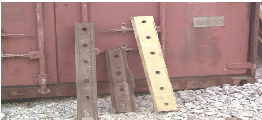
Figure 1.6: Three basic types of rail joints[29].
